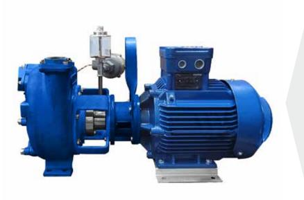
Suction port Threaded - 1 1/2" ISO 228 (BSP) Delivery port Threaded - 1 1/2" ISO 228 (BSP) Qmax 24 m<sup>3</sup>/h - 400 l/min (105 USgpm) Hmax 16 m (52 ft) Solids handling 20 mm (0.8") Motor power 1,1 kW - 1,5 HP Motor type **IEC** standard **Cast iron frame** Motor brand CEMP Weight 47 kg (104 lb)
